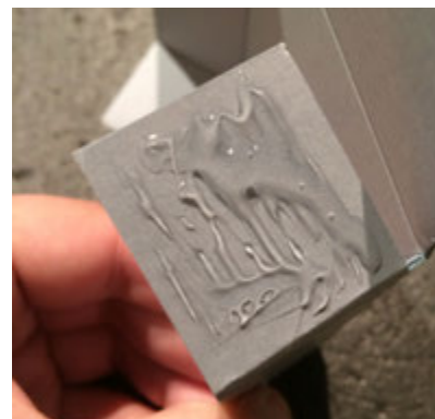
The right amount of glue – the glue is spread out evenly
