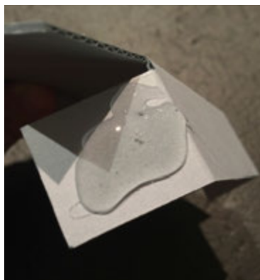
Too much glue – the excess glue may ooze out
